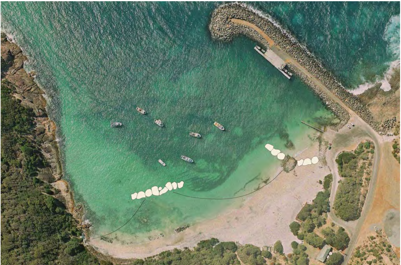
Figure 16: Rubble mound cut-off groyne to be constructed near boat ramp in combination with an offshore breakwater at the western end of the beach to create a buffer in front of the erosion-susceptible western dune.
