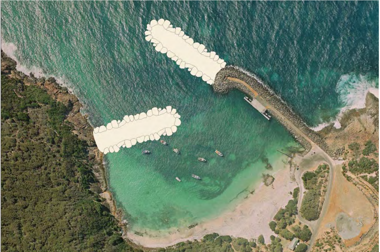
Figure 17: Major harbour construction works, including the extension of the original breakwater into deeper water, and the construction of a new spur-type breakwater from the western granite headland. This would effectively shelter the entire beach inside the harbour.
