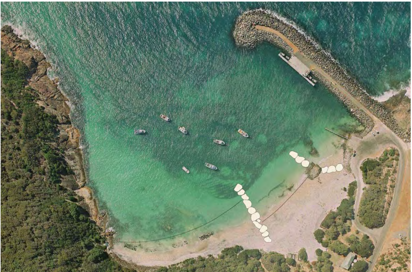
Figure 15: Rubble mound cut-off groyne to be constructed near boat ramp in combination with a geotextile bag mid-beach groyne to compartmentalise Fishery Beach to ensure stability.
