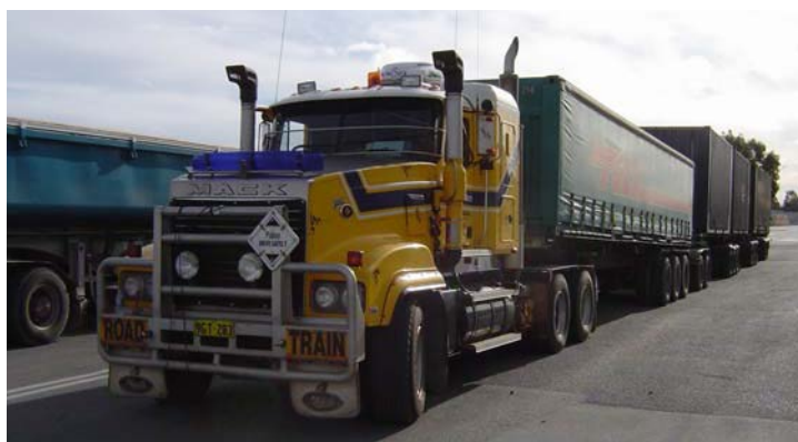
Figure 13 A+B3 container combination
