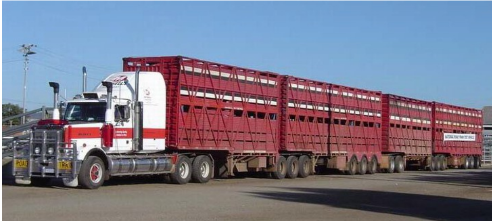
Figure 11 BAB-quad livestock combination
