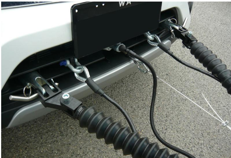
**Figure 5.** correct example of A-frame attachment
