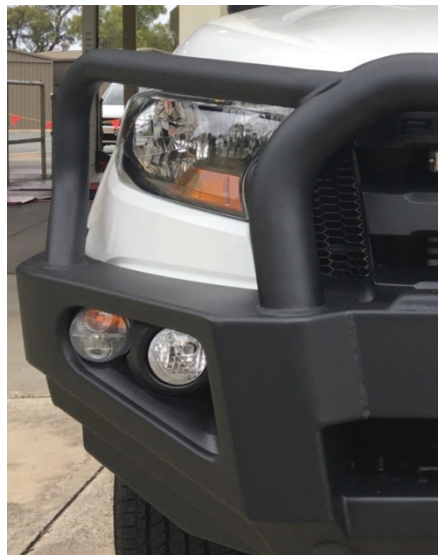
Figure 8 - Examples of acceptable additional lighting on an FPS.
