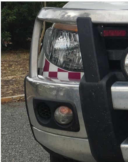
Figure 8 - Examples of acceptable additional lighting on an FPS.
