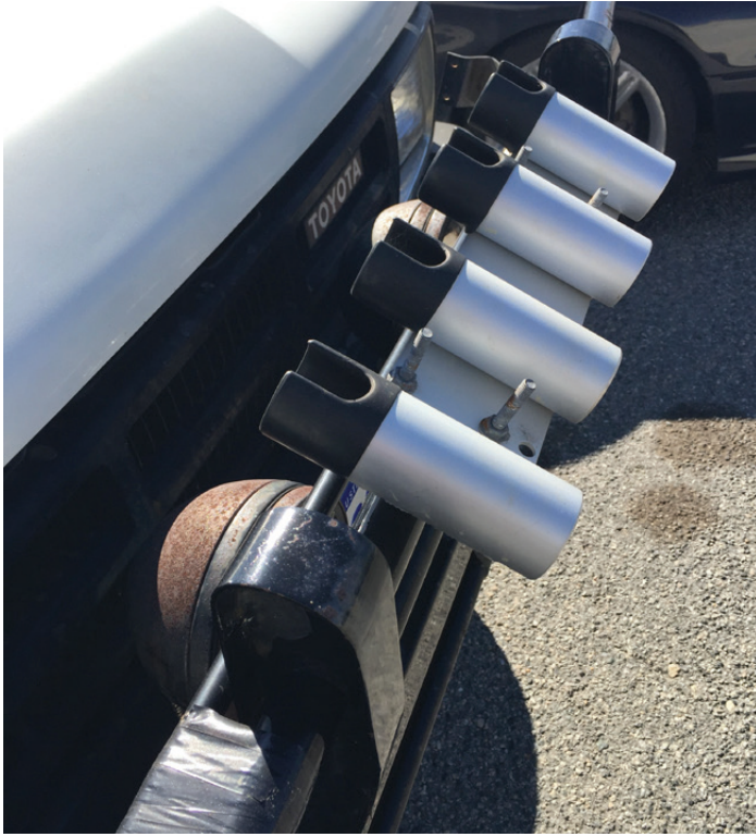
Figure 7 - A rod holder mounted as shown is a dangerous projection and is not acceptable.
