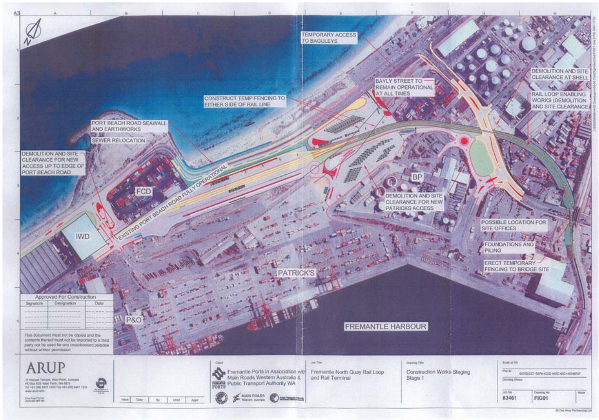
Figure 11 Stage 1 Construction Works for Fremantle Inner Harbour Rail Access
