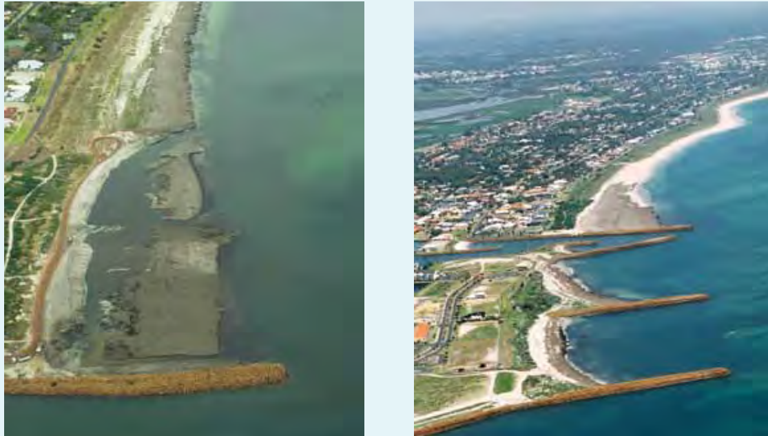
Figure 1 Typical accumulation of wrack a) adjacent to the western training wall and b) Moonlight Bay.
