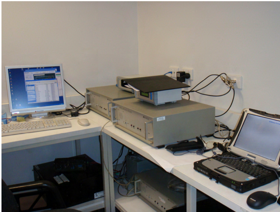
Figure 12. Shore receiving station for the Rottneest wave buoy at the Marine Operations Centre.
