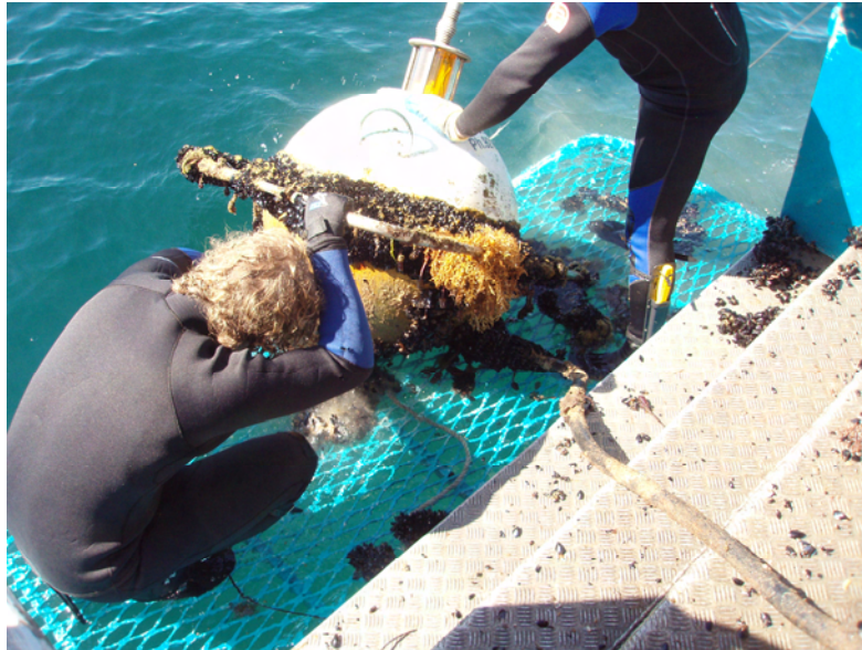
Figure 9. Typical biofoul found on a buoy after 12 months of deployment.
