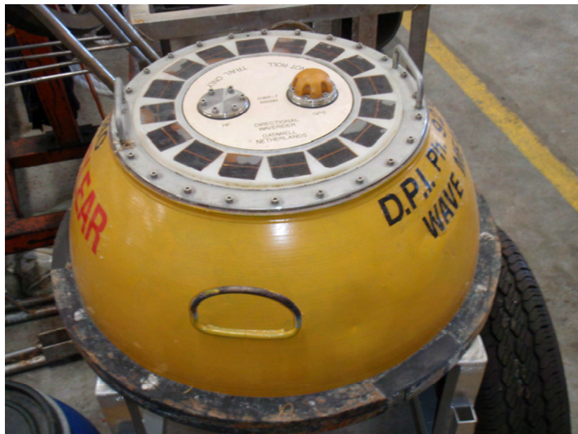
Figure 8. Instrumentation found on top of a directional wave buoy including solar panels and connections for the data transmitting antenna.
