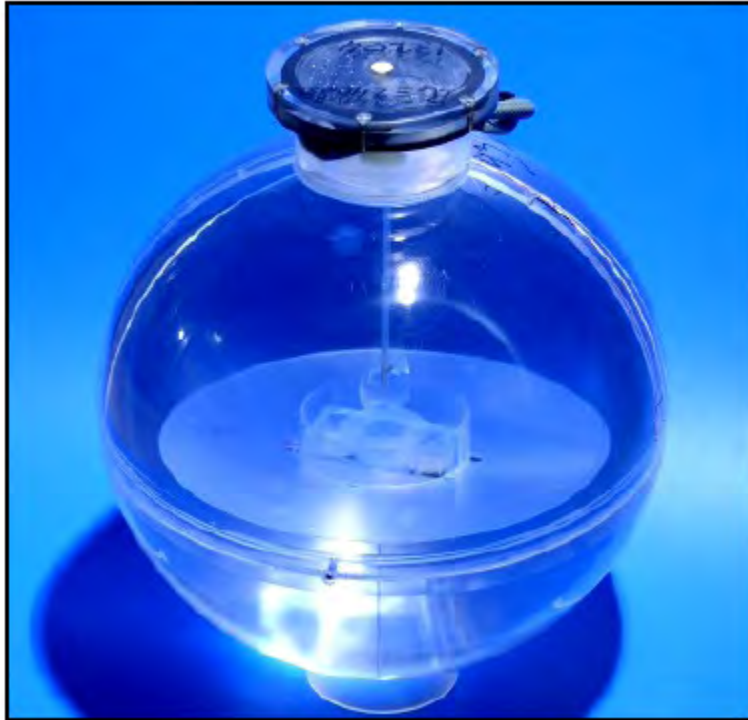
Figure 7. Datawell stabilised platform motion sensor. This is a fluid filled sphere allowing the motion sensor to be perfectly buoyant (Datawell 2008).
