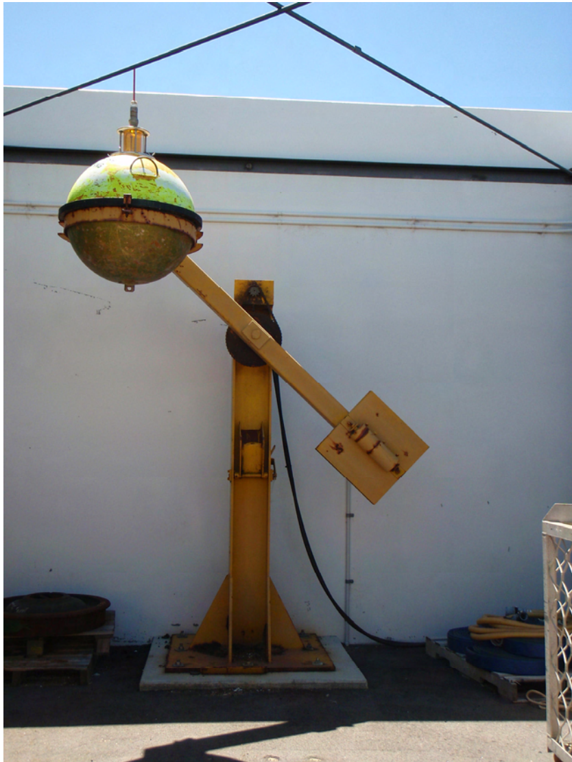
Figure 2. Wave buoy calibration using the calibration arm at DPI's Marine Operations Centre to simulate a 2 m wave.
