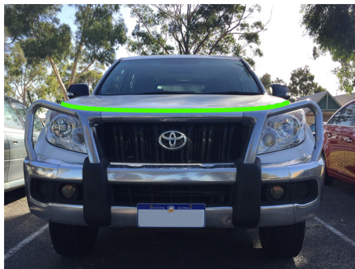
Figure 2 - Example of upward trajectory of FPS.
