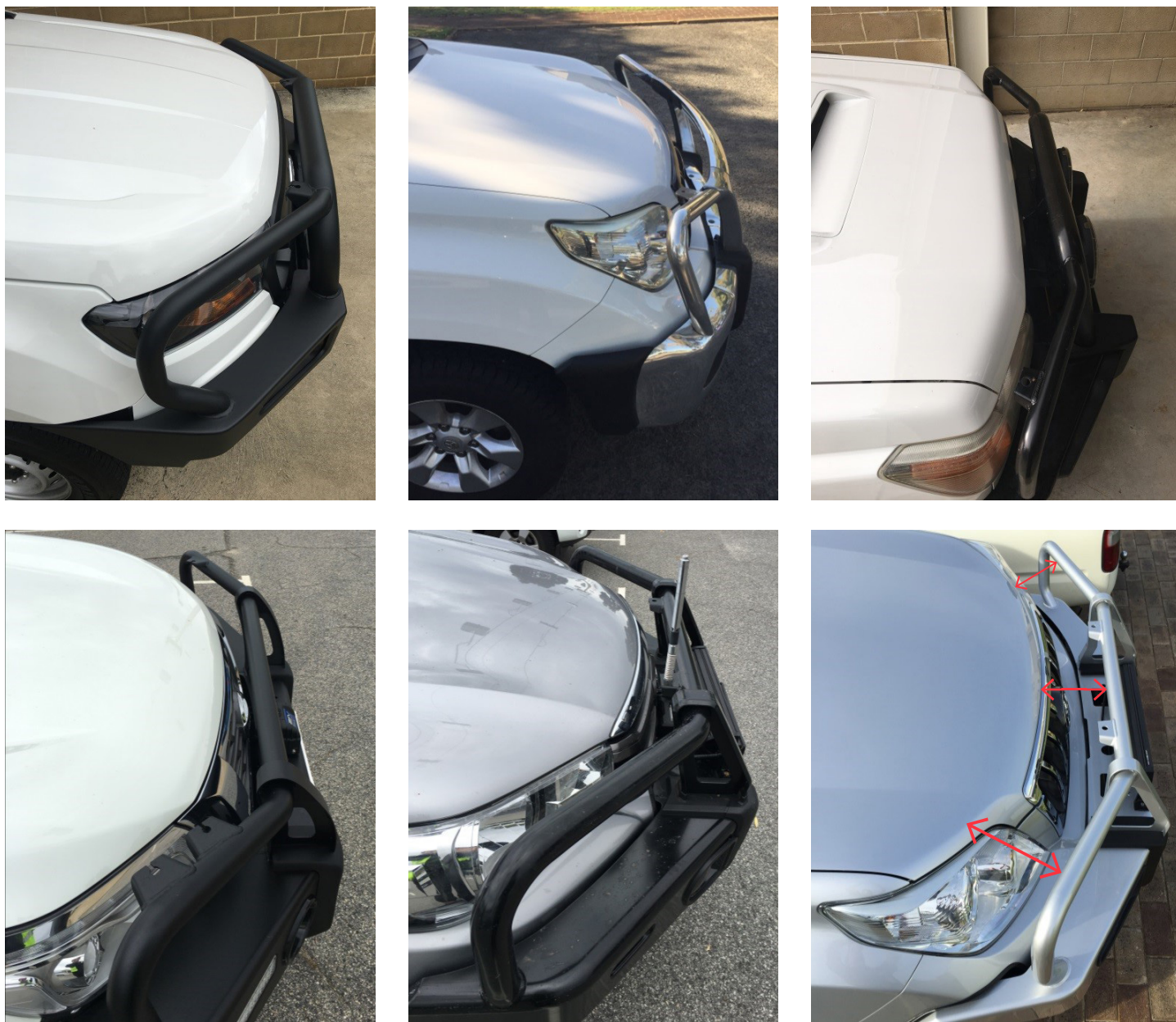
Figure 3 - Examples of acceptable FPS designs.
