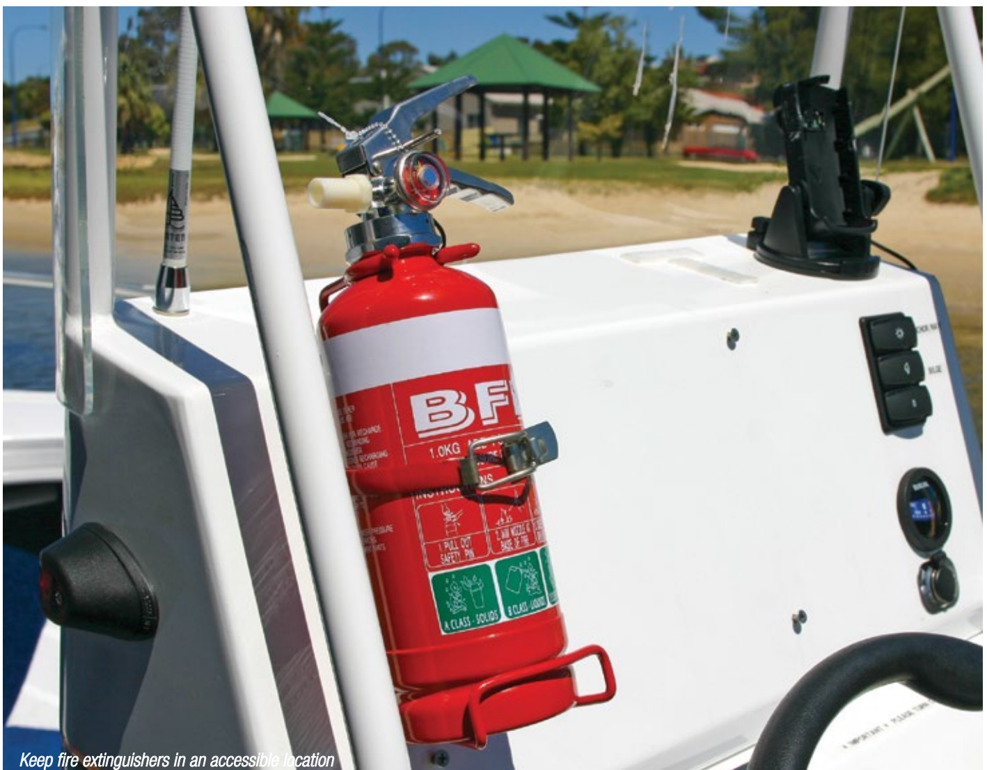
Check the gauge is in the green
