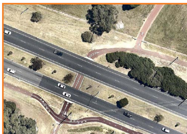
Figure 4.23 Shared paths which cross busy dual carriageway roads do not necessarily require expensive solutions such as underpasses or traffic signals. Sufficiently wide refuges can help people safely stagger their crossings.
