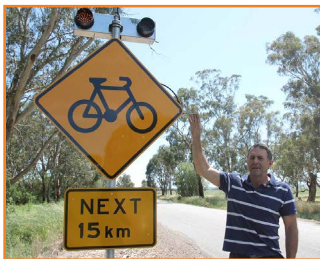
Figure 4.29 Button-activated warning lights could help further improve cyclist safety along the Wolf Pack Route.
