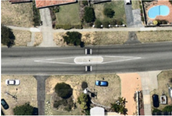
Figure 26: Single lane angled slow point.
