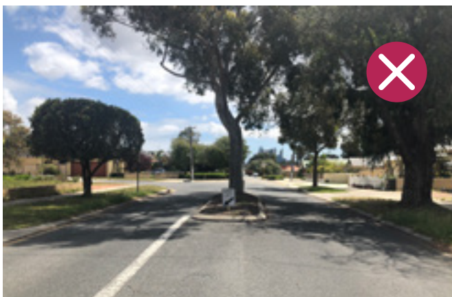
(b) Two lane parallel slow point - Lacks visual obstruction
