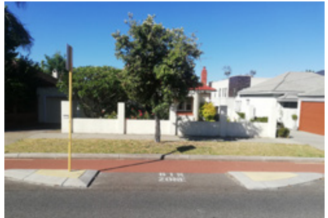
Figure 11: Example placement of a bin zone adjacent to a cycle bypass or bike lane.
