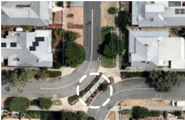
Figure 41: Diagonal road closure
