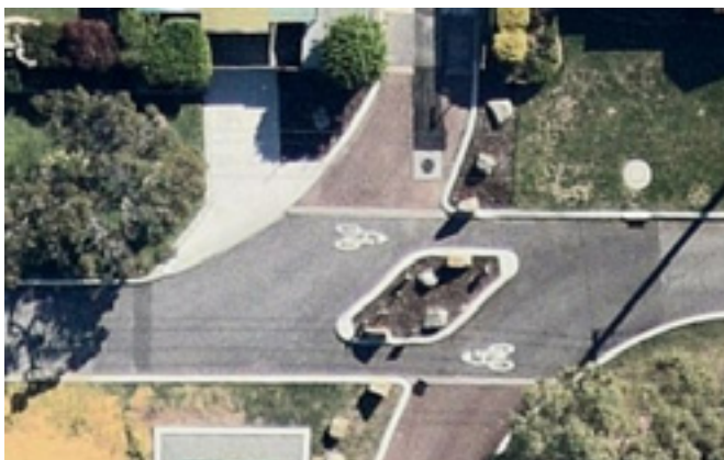
Figure 42: Diagonal road closure
