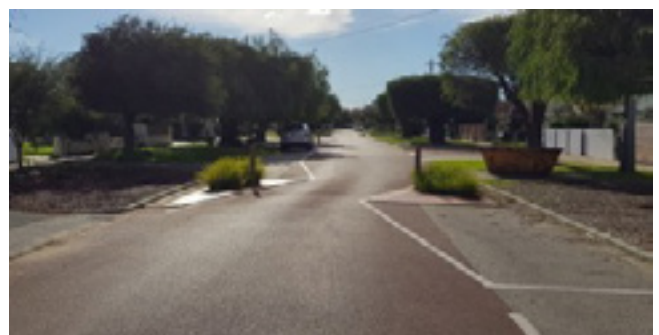
Figure 28: Typical single lane angled slow point.
