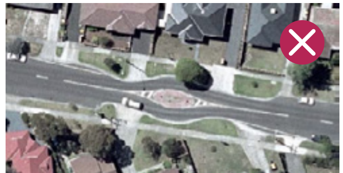
Figure 15: Centre Blister Island treatment on wider carriageway.
