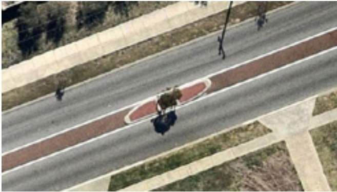
Figure 53: Raised central median.
