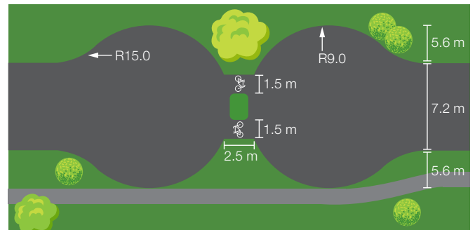
Figure 39: Mid-block (full closure).
