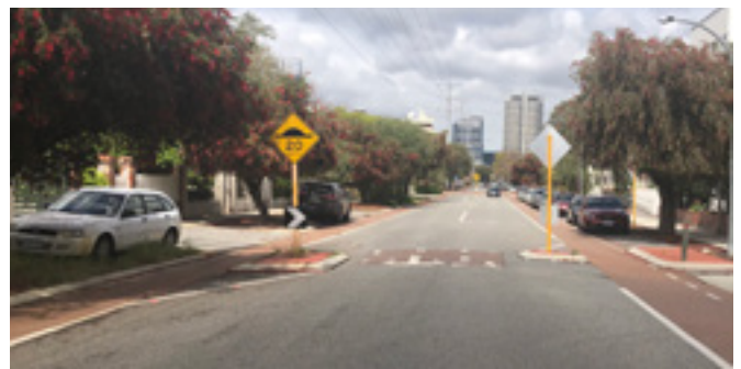
Figure 27: Single lane parallel slow point.
