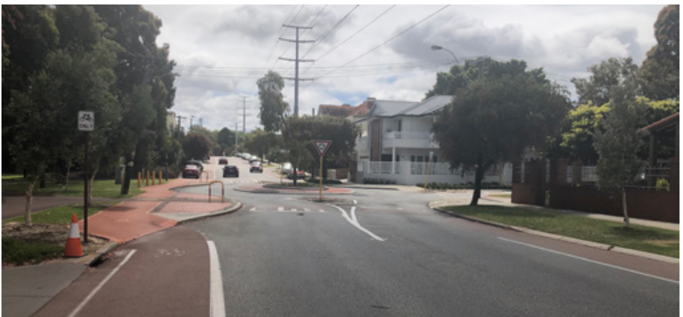
Figure 62: Transition ramp at roundabout for riders to merge onto shared path.
