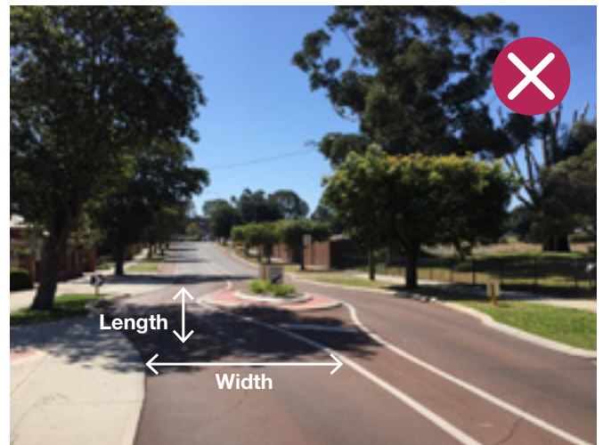
Figure 14: Centre blister island treatment on narrow carriageway.
