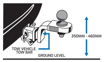
The most commonly used 50 mm diameter tow balls are not rated beyond 3,500 kgs. Towing 3,500 kgs to 4,500 kgs requires the use of a 75 mm tow ball or other coupling rated to the ATM of the trailer.
