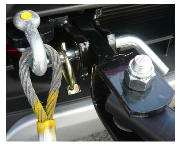
Figure 1. example of correct connection
