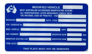
The attachment of the modification plate is essential as this represents the CEO's approval to modify. Where no VSB6 plate is attached a vehicle requires the issue of a modification permit.
