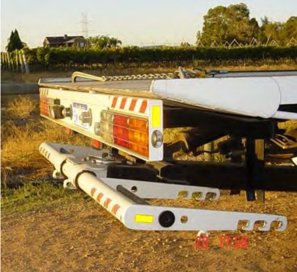
Light bar in normal position
