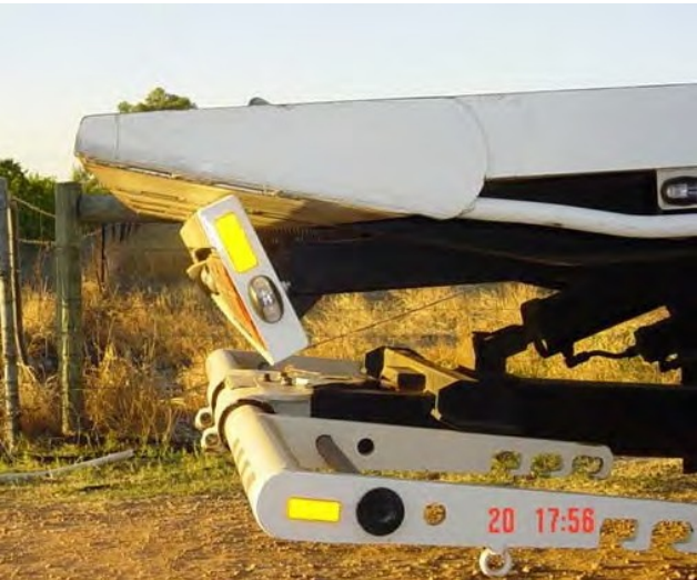
Light bar tilts as tray begins to move rearwards
