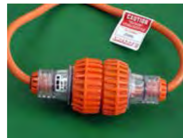
Joint in supply leads: Comprising IP56 plug and socket
