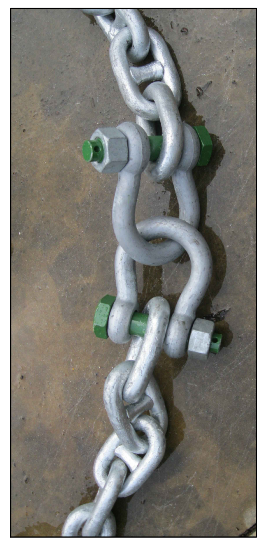
2 DETAIL - SPLICING LENGTH OF CHAIN TO SLAC (12 No. INCLUDING 1 SPARE) 8-1 NTS
