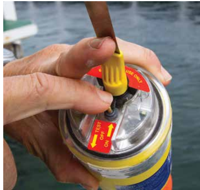
Regularly use the test switch to check your distress beacon is in working condition.
