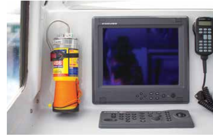
Store distress beacons in an accessible place.
