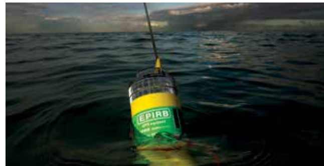
An EPIRB is designed to float in water.
