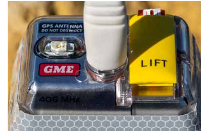
GPS antenna need to have a clear view of the sky
