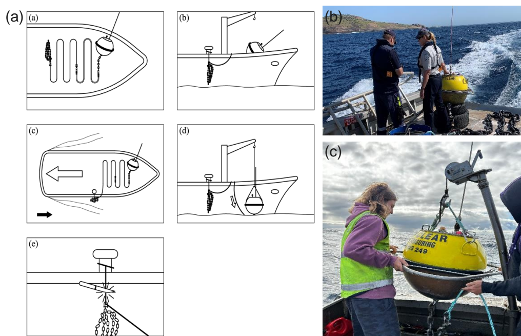
Figure 8. Buoy deployment: (a) Diagram illustrating the procedure (Datawell, 2017); (b) Buoy onboard at Bremer Bay before deployment; (c) Buoy deployment in progress.
