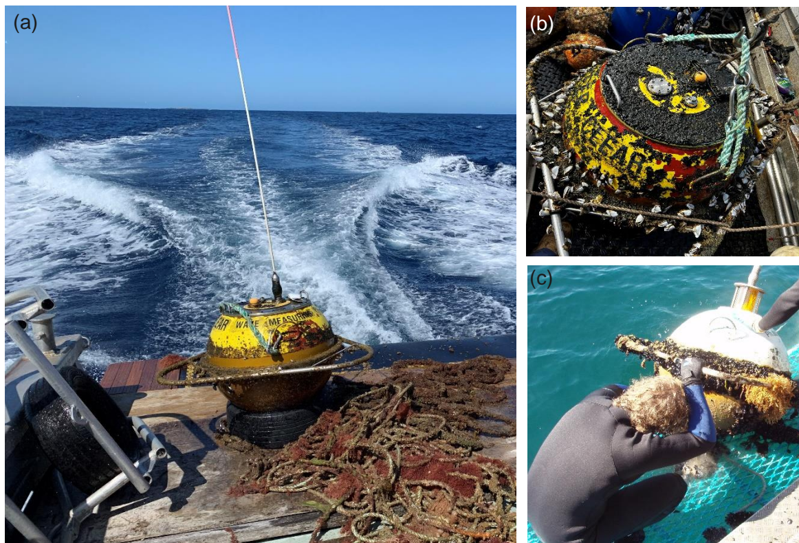
Figure 9. Recovery of the DoT buoy: (a) Buoy onboard after recovery; (b) Buoy covered with biofouling after recovery at Bremer Bay; (c) Removal of biofouling.
