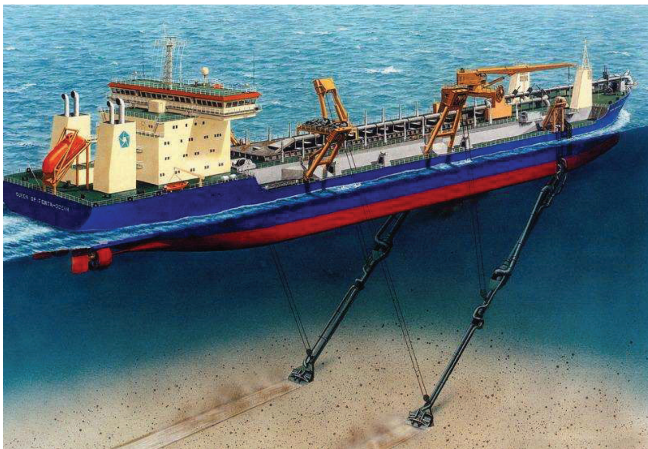
Figure 3-2 Trailer suction hopper dredge (confluence.qps.nl, 2021)
