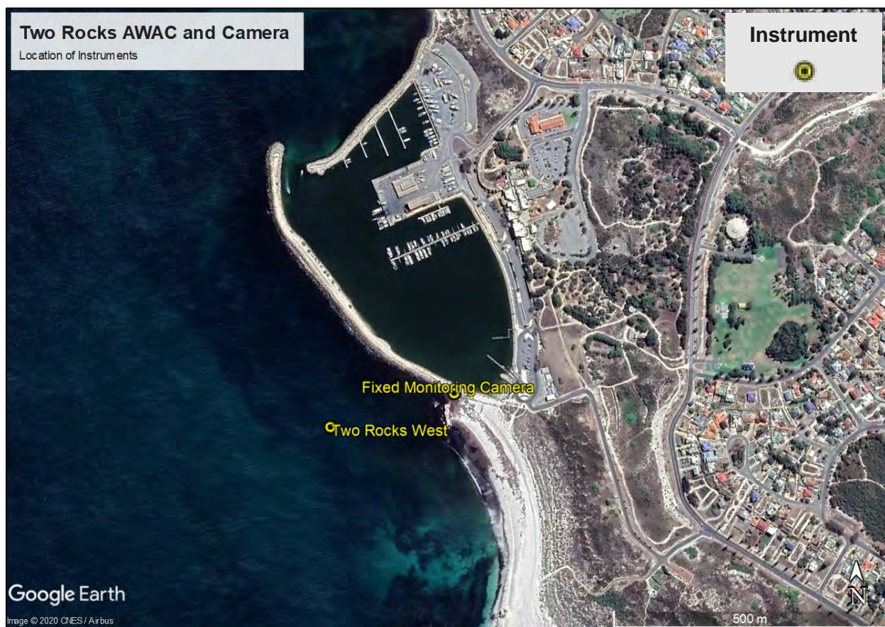
Figure 1: Two Rocks West AWAC location (31.4994° S, 115.5808° E) and Fixed Monitoring Camera location (31.4988° S, 115.5832° E); the deployed AWAC depth was approximately 5m.
