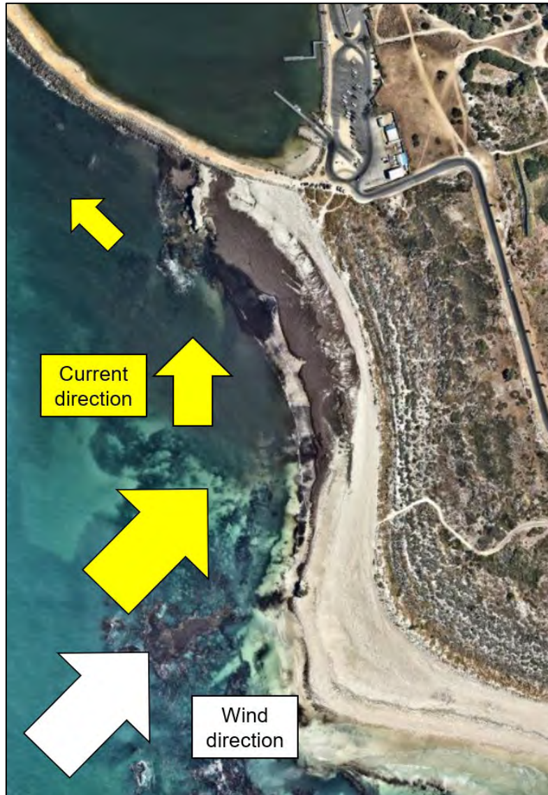
Figure 19: Conceptual model of current circulation patterns expected during a Seabreeze event, smaller arrows present anticipated weakening currents as they encounter friction with the shore
