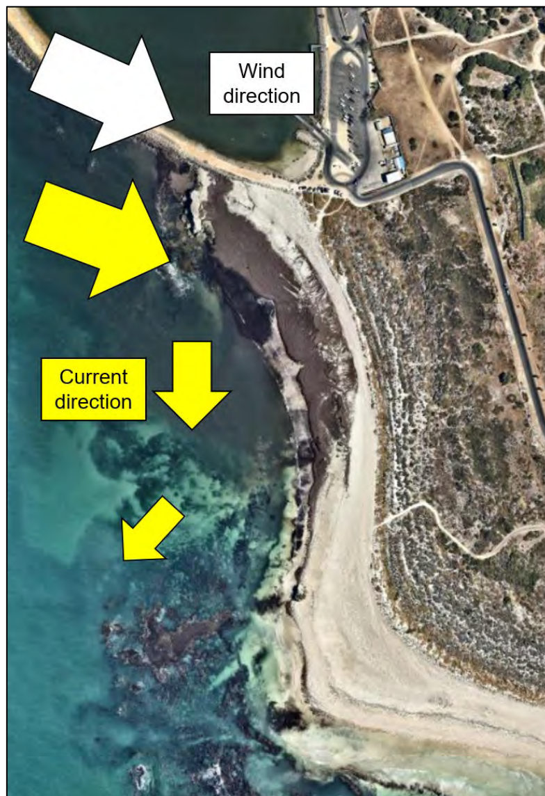
Figure 22: Conceptual model of current circulation patterns expected during a Storm event, smaller arrows present anticipated weakening currents as they encounter friction with the shore
