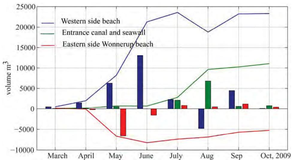
**Figure 4.81 Model-simulated monthly sand accretion and cumulative volume from 1 March to 30 October 2009 at different locations across Port Geographe for Scenario 7.**
