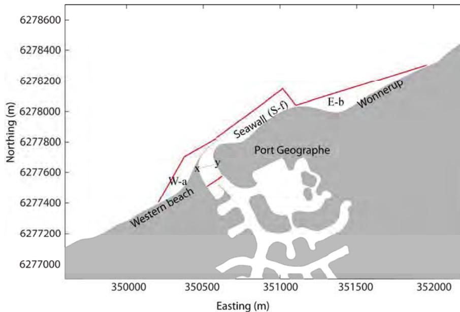
**Figure 4.37** Areas selected to estimate accretion/erosion of sand and seagrass wrack for Scenario 2. W-a (western beach), S-f (front of seawall) and E-b (Wonnerup). Cross-section x-y at the harbour entrance was selected to evaluate bed level changes.
