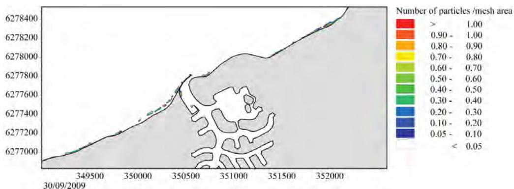
**Figure 4.44 Model-simulated particle distribution for Scenario 2 in the vicinity of Port Geographe on 30 September 2009.**
