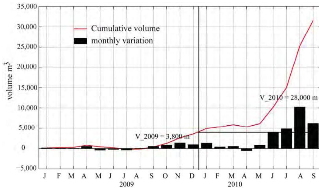
**Figure 4.20 Predicted monthly sand accretion (black bar) and cumulative sand volume (red line) from January 2009 to 30 September 2010 within the groyne fields and the harbour entrance.**
