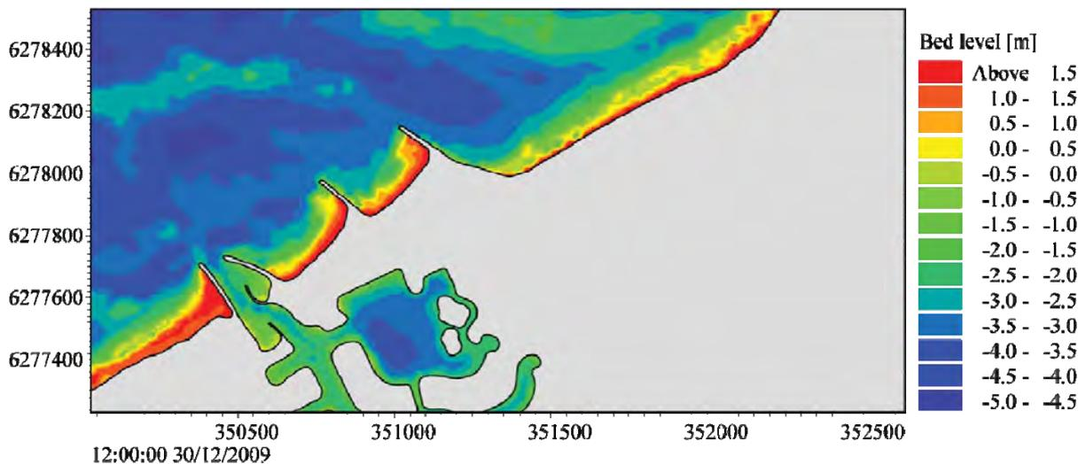
**Figure 4.14 Model-predicted bed levels in the vicinity of Port Geographe on 30 December 2009 (The initial bathymetry used for the 2010 model run).**
