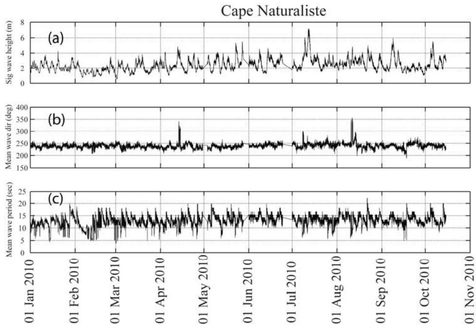
**Figure 4.7** Open boundary wave climate forcing data in 2010, obtained from the Cape Naturaliste Wave Buoy (source: Western Australian Department of Transport). (a) Significant wave height, (b) mean wave direction and (c) mean wave period.
