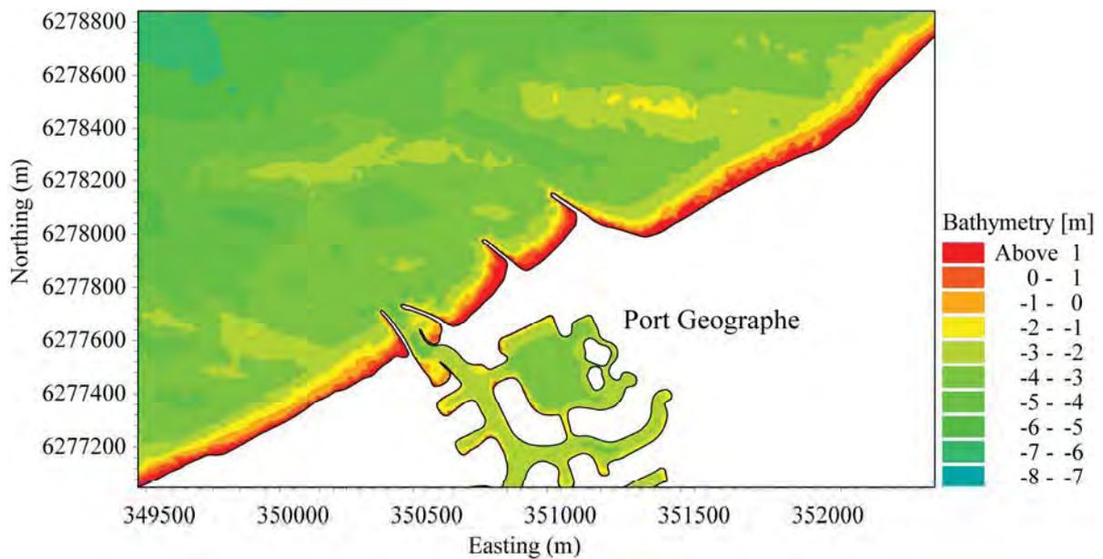
Figure 2.4: Initial model bathymetry of Port Geographe and Wonnerup areas in the existing configuration.
