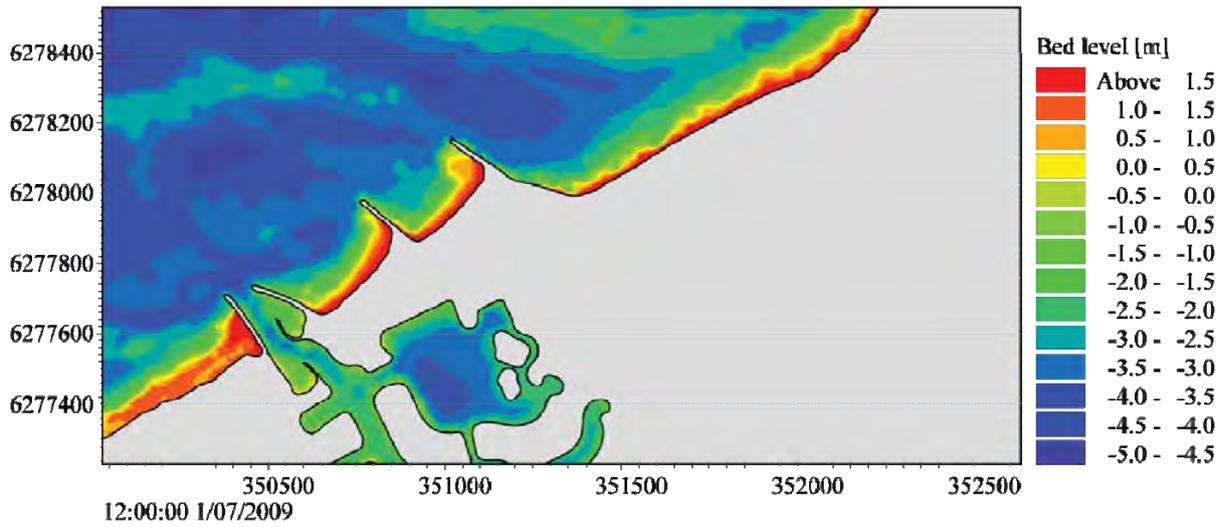
Figure 3.17 Model-predicted bed levels in the vicinity of Port Geographe on 1 July 2009.
