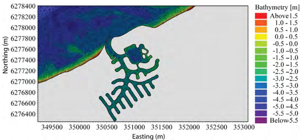
Figure 4.46 Scenario 3 mesh grid and initial model bathymetry of Port Geographe including all inner canal segments.
