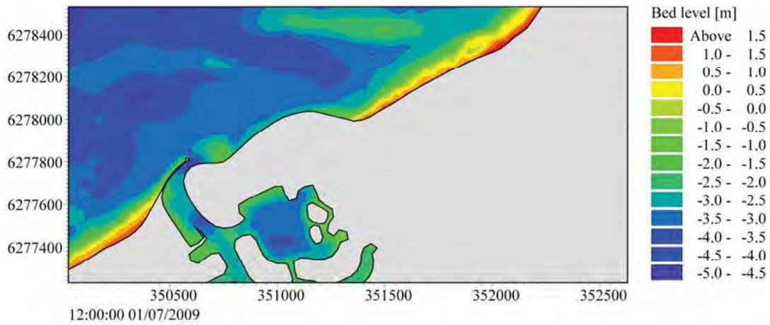
**Figure 4.34 Model-predicted bed levels in the vicinity of Port Geographe for Scenario 2 on 01 July 2009.**
