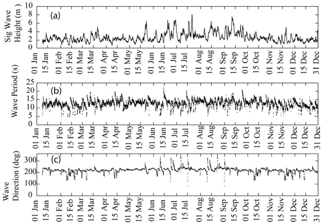
**Figure 2.9** Open boundary wave climate forcing data for 2009, obtained from the Cape Naturaliste Wave Buoy and the Global Wave-Watch III wave model: (a) Significant wave height, (b) Mean wave period and (c) Mean wave direction.
