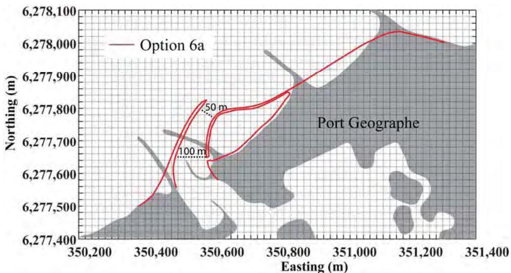
**Figure 4.77 Scenario 7 layout of Port Geographe. Black dotted line shows existing Port Geographe layout and red solid lines shows layout of Scenario 7.**
