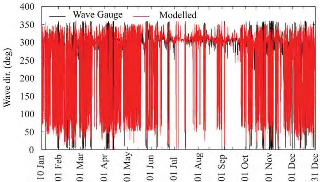
**Figure 3.8 Measured and predicted mean wave direction at the AWAC site in 2009. Black lines denote observed data and red lines denote model output.**
