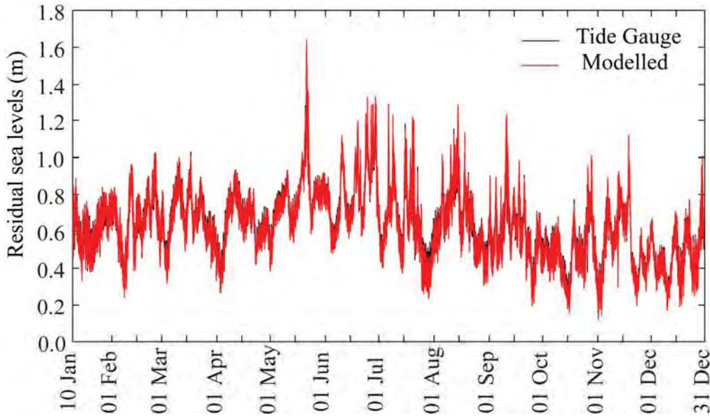
**Figure 3.3 Measured and predicted residual sea levels at the Busselton tide station in 2009. Black lines denote observed data and red lines denote model output.**
