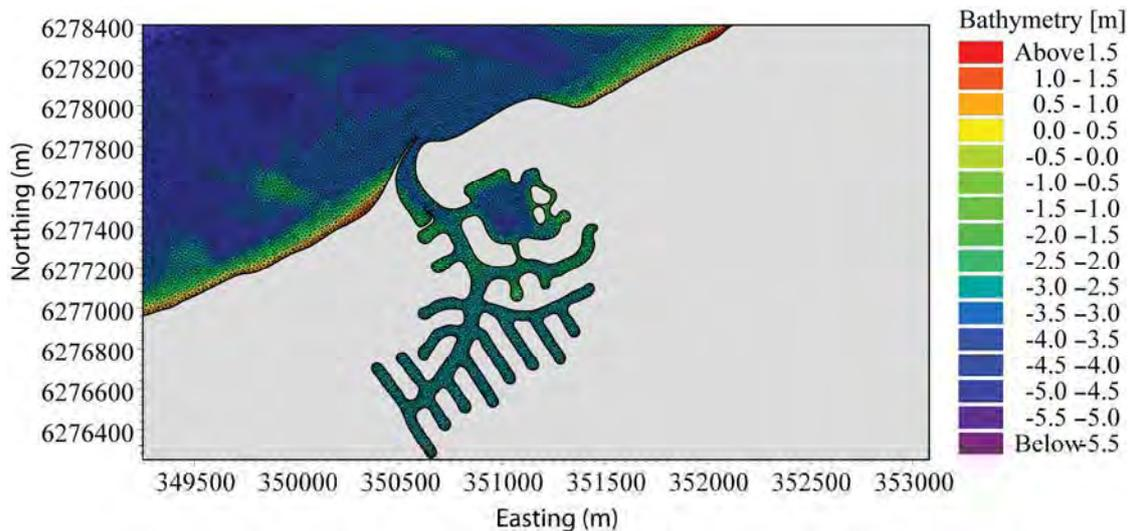
**Figure 4.54 Mesh grid and bathymetry in the vicinity of Port Geographe for Scenario 4 including all inner canal segments.**
