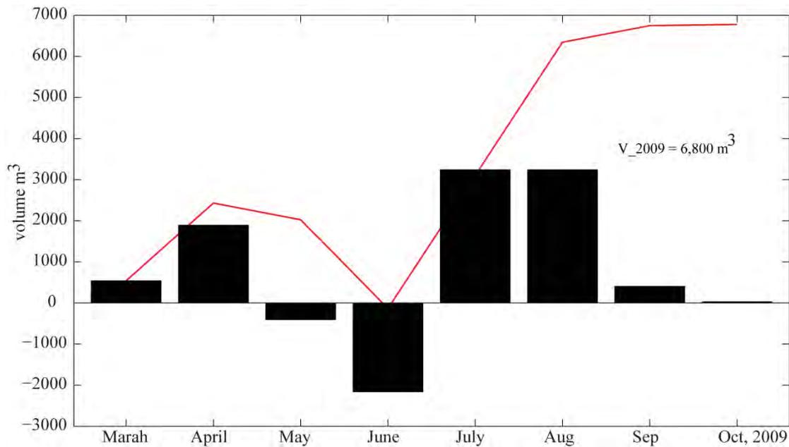
**Figure 4.41 Predicted monthly sand accretion and cumulative sand volume from 1 March to 1 November 2009 along the eastern side of the harbour entrance (see Figure 4.37 for selected area) beach under Scenario 2.**
