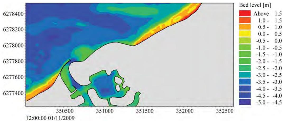
**Figure 4.36 Model-predicted bed levels in the vicinity of Port Geographe for Scenario 2 on 1 November 2009.**
