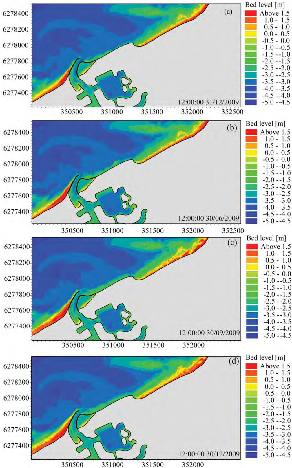
**Figure 4.93 Model-predicted bed levels in the vicinity of Port Geographe for scenario 8 with initial saturated beach on the western side of Port Geographe. (a) Model initial bathymetry on 31 Dec 2009, and predicted bed levels on (b) 30 June 2009; (c) 30 September 2009; and, (d) 30 December 2009**
