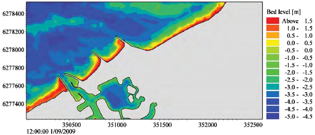
**Figure 3.19 Model-predicted bed levels in the vicinity of Port Geographe on 1 September 2009.**
