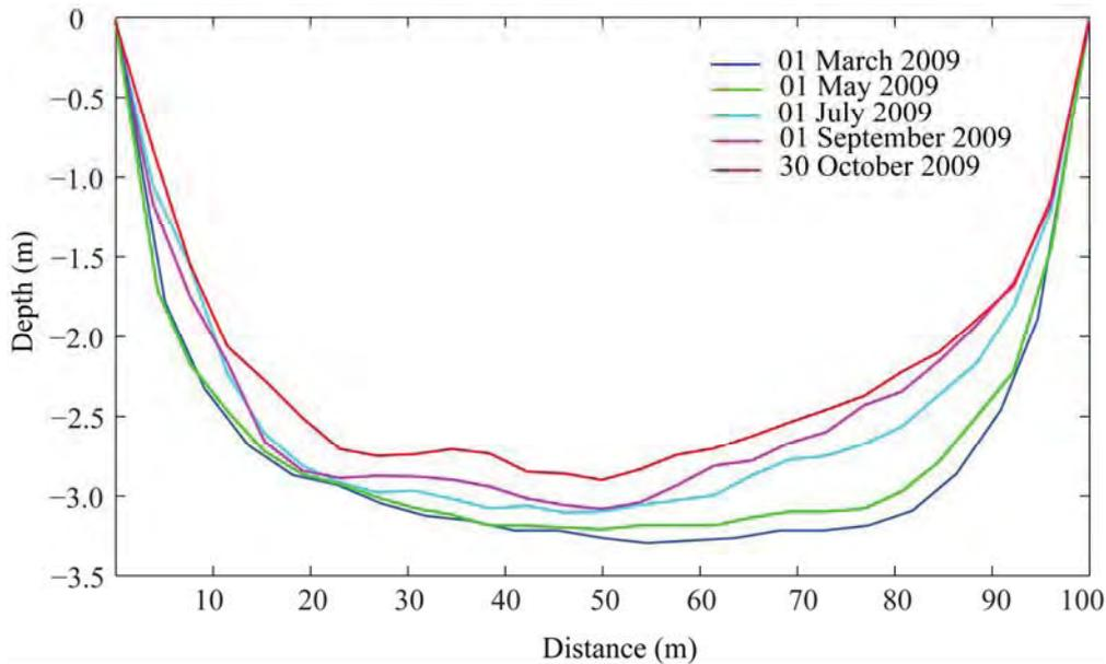
**Figure 4.64 Model-predicted bed levels across the harbour entrance channel (section x-y) of Port Geographe for Scenario 5 during 01 March to 30 October 2009.**
