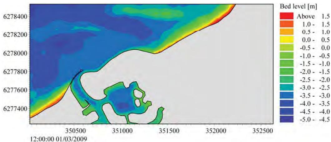
**Figure 4.32 Model initial bed levels in the vicinity of Port Geographe for Scenario 2 on 01 March 2009.**
