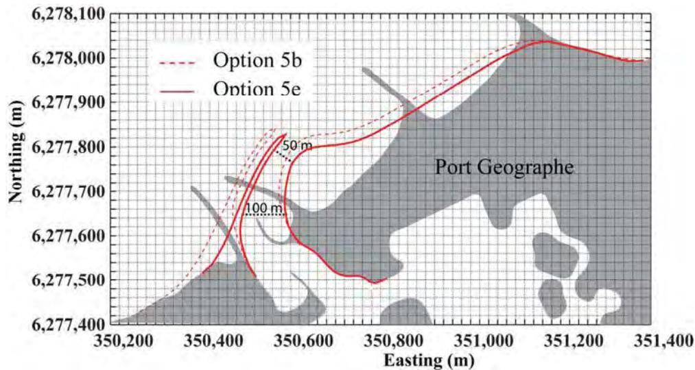
**Figure 4.69 Scenario 6 layout of Port Geographe. Black dotted line shows existing Port Geographe layout, red dotted line shows layout of Scenario 3 and red solid line shows layout of Scenario 6.**
