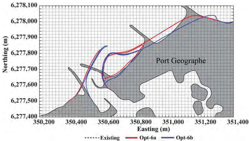
**Figure 4.2: Layouts for scenarios 7 and 8 with the inclusion of a small lagoon behind the seawall.**
