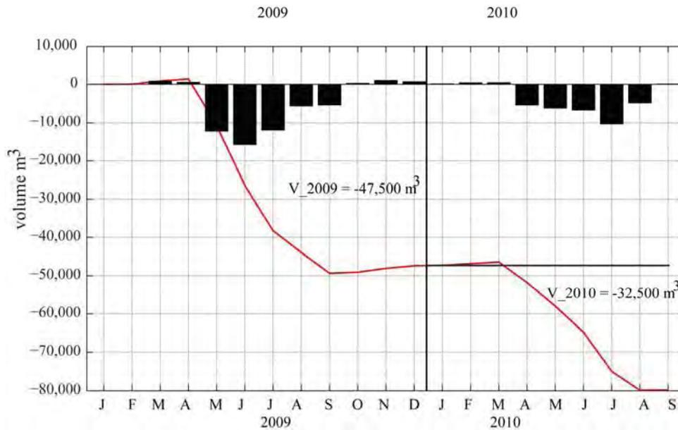
**Figure 4.21 Predicted (negative) monthly sand accretion (black bars) and cumulative (red line) sand volume from January 2009 to 30 September 2010 on the eastern beach (Wonnerup). (Note: negative values signify erosion).**
