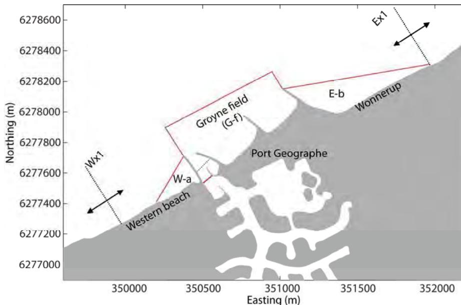
**Figure 4.18 Map showing areas used to calculate the sand budget. W-a (western beach); G-f (Port Geographe foreshore); and, E-b (Wonnerup foreshore). Cross-sections to predict bedload sand transport are shown as Wx1 (western section) and Ex1 (eastern section).**
