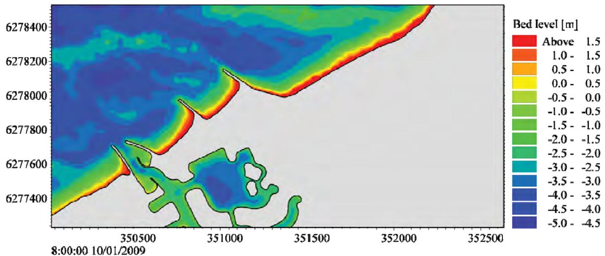
Figure 3.11 Model initial bed levels (bathymetry) in the vicinity of Port Geographe.
