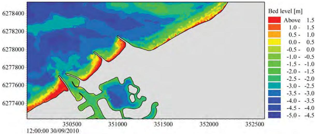
**Figure 4.17 Model-predicted bed levels in the vicinity of Port Geographe on 30 September 2010.**
