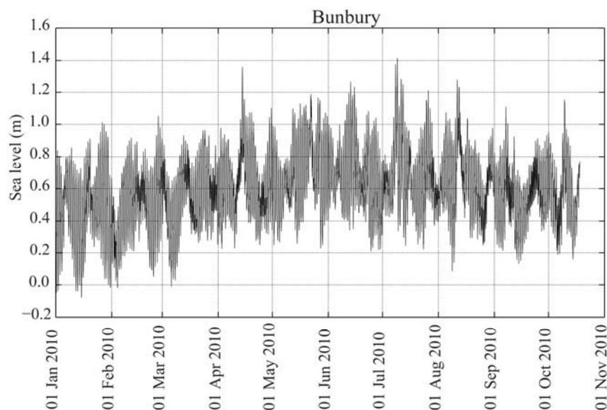
**Figure 4.3 Open boundary water level forcing data in 2010 from the Bunbury tide gauge (source: Western Australian Department of Transport).**
