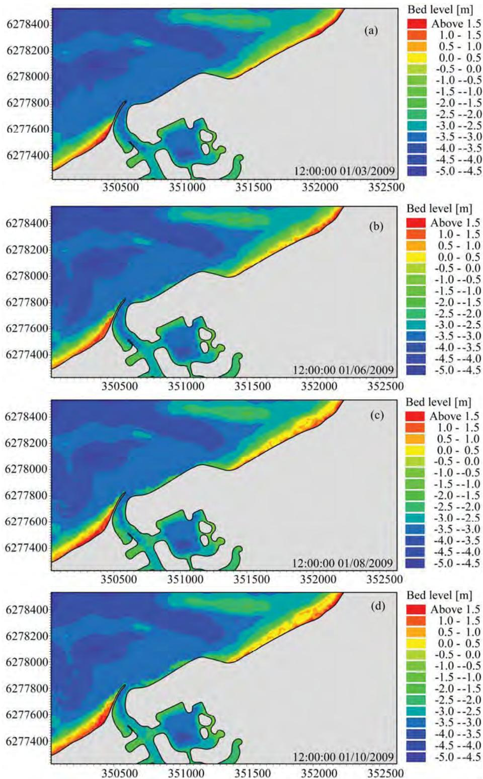
**Figure 4.71 Model-predicted bed levels in the vicinity of Port Geographe for Scenario 6. (a) Model initial bathymetry on 01 March 2009 and predicted bed levels on (b) 1 June 2009; (c) 01 August 2009; and, (d) 01 October 2009**
