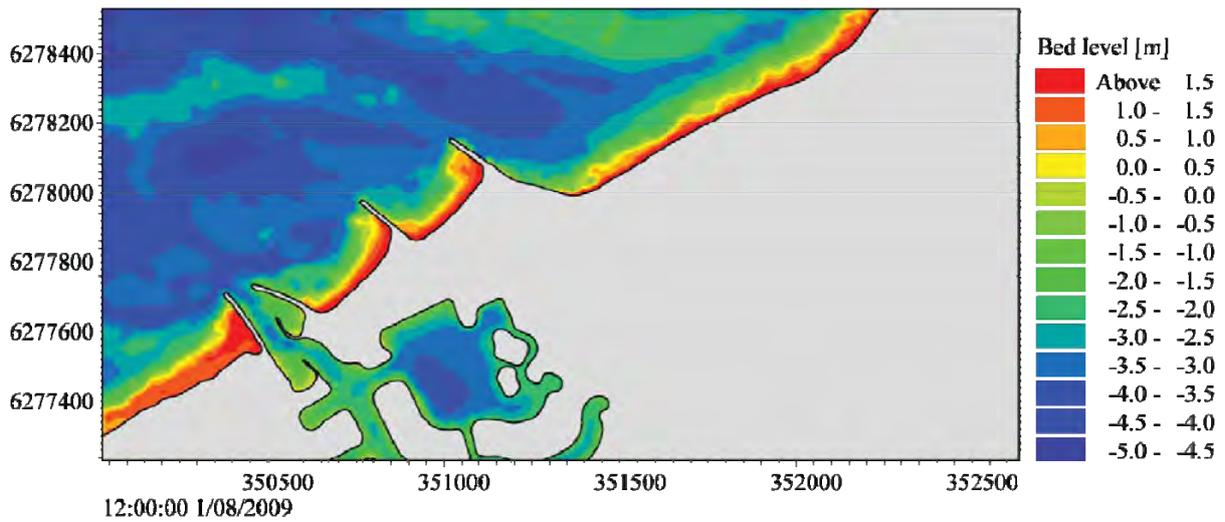
Figure 3.18 Model-predicted bed levels in the vicinity of Port Geographe on 1 August 2009.
