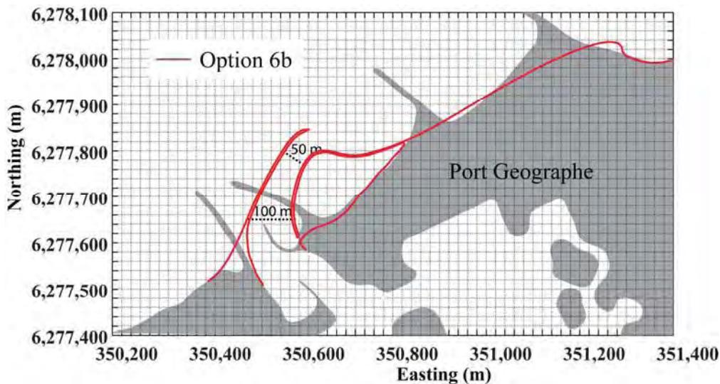
**Figure 4.85 Scenario 8 layout of Port Geographe. Black dotted line shows existing Port Geographe layout and red solid lines shows layout of Scenario 8.**
