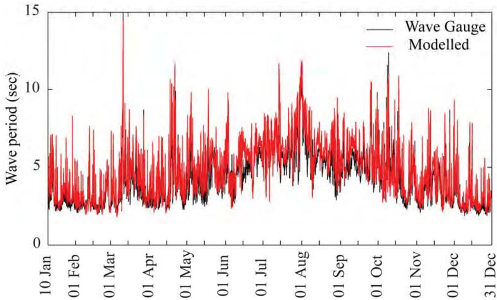
**Figure 3.9 Measured and predicted mean wave periods at AWAC site in 2009. Black lines denote observed data and red lines denote model output.**
