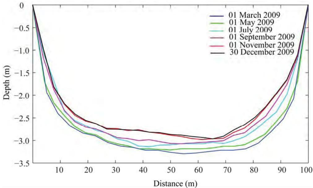
**Figure 4.88 Model-predicted bed levels across the harbour entrance channel (section x-y) of Port Geographe for Scenario 8 during 01 March to 30 December 2009.**
