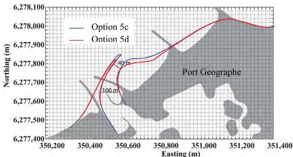
**Figure 4.61 Layout for Scenario 5 at Port Geographe. Blue line shows Scenario 4 - layout and the red line shows the layout for Scenario 5.**
