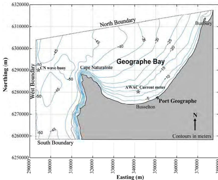
**Figure 2.2 Map of Geographe Bay showing the model boundaries, general bathymetry and the locations of model input data (tide gauge, wave gauge, current meter, and the meteorological stations at Cape Naturaliste, Busselton and Bunbury).**
