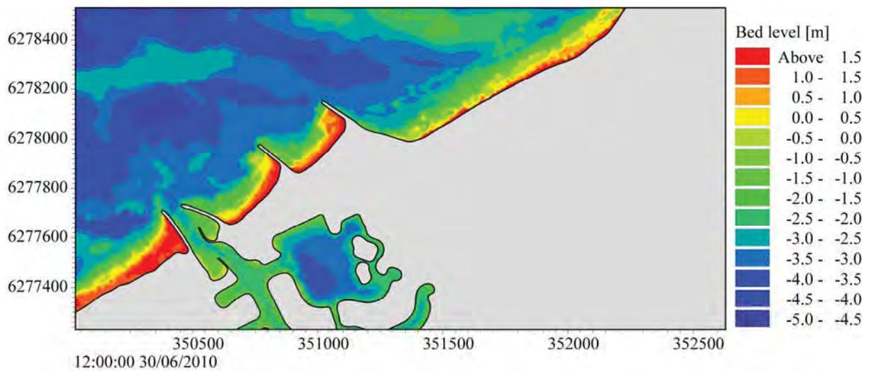
**Figure 4.16 Model-predicted bed levels in the vicinity of Port Geographe on 30 June 2010.**
