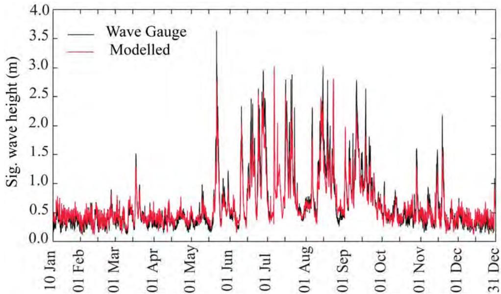
**Figure 3.7 Measured and predicted significant wave height at the AWAC site in 2009. Black lines denote observed data and red lines denote model output.**
