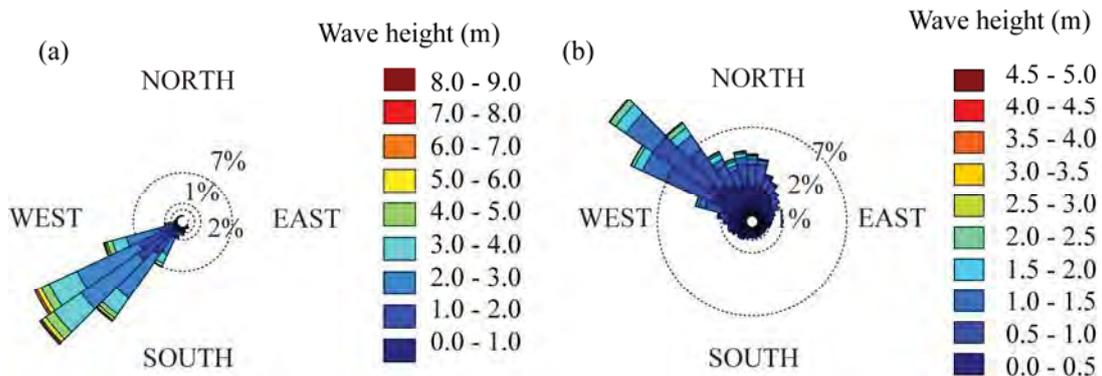
**Figure 2.10** Wave rose diagrams showing predominant wave climate at (a) Cape Naturaliste; and, (b) AWAC site at Busselton (wave heights are in m).
