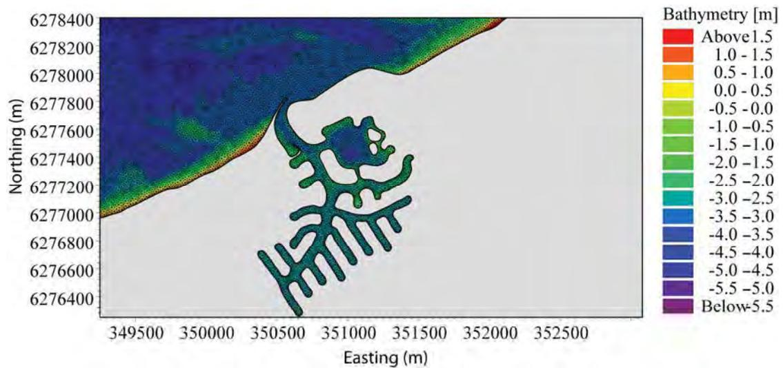
**Figure 4.62 Mesh grid and initial bathymetry in the vicinity of Port Geographe for Scenario 5 including all inner canal segments.**
