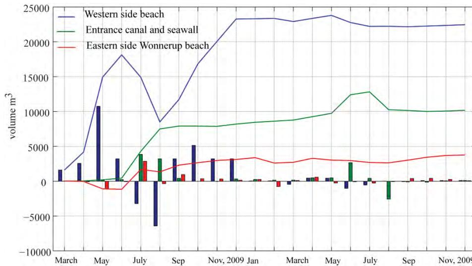
**Figure 4.94 Model-simulated monthly sand accretion and cumulative volume during 01 March 2009 to December 2009 and repeat January 2009 to December 2009 at different part of Port Geographe for scenario 8.**
