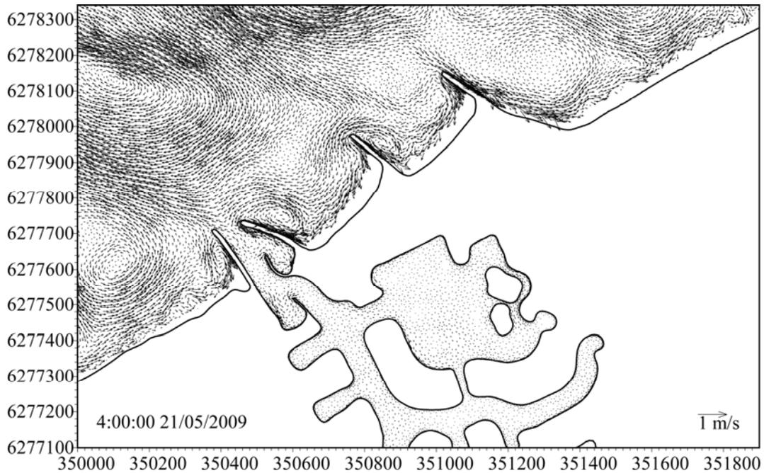
**Figure 4.10** Predicted velocity vectors in the vicinity of Port Geographe during storm event (0400 hrs, 21 May 2009).
