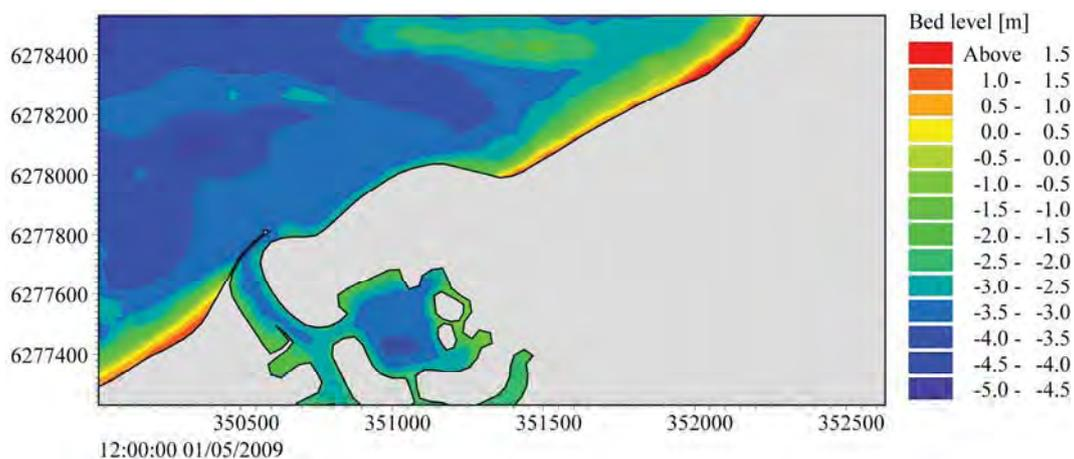
**Figure 4.33 Model-predicted bed levels in the vicinity of Port Geographe for Scenario 2 on 01 May 2009.**
