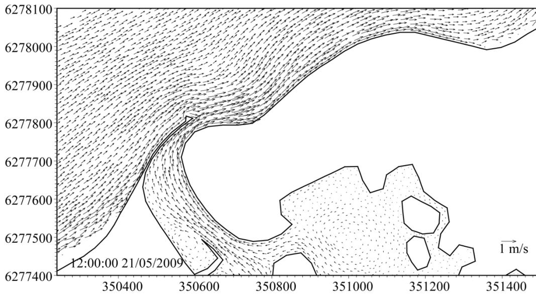
**Figure 4.31 Model-predicted current pattern in the vicinity of Port Geographe for Scenario 2 (Option 5a) at peak of storm event (1200 hr, 21 May 2009).**
