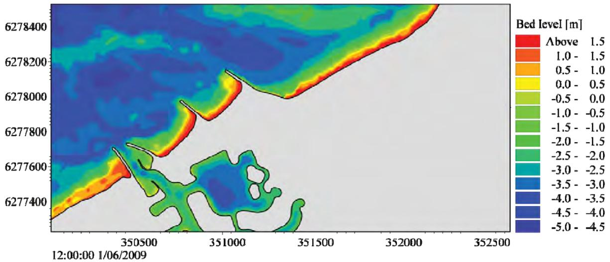
Figure 3.16 Model-predicted bed levels in the vicinity of Port Geographe on 1 June 2009.
