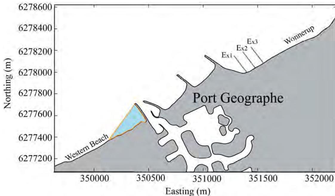
**Figure 3.24 Port Geographe: area selected (light blue) to estimate accretion/erosion of sand along the western beach.**
