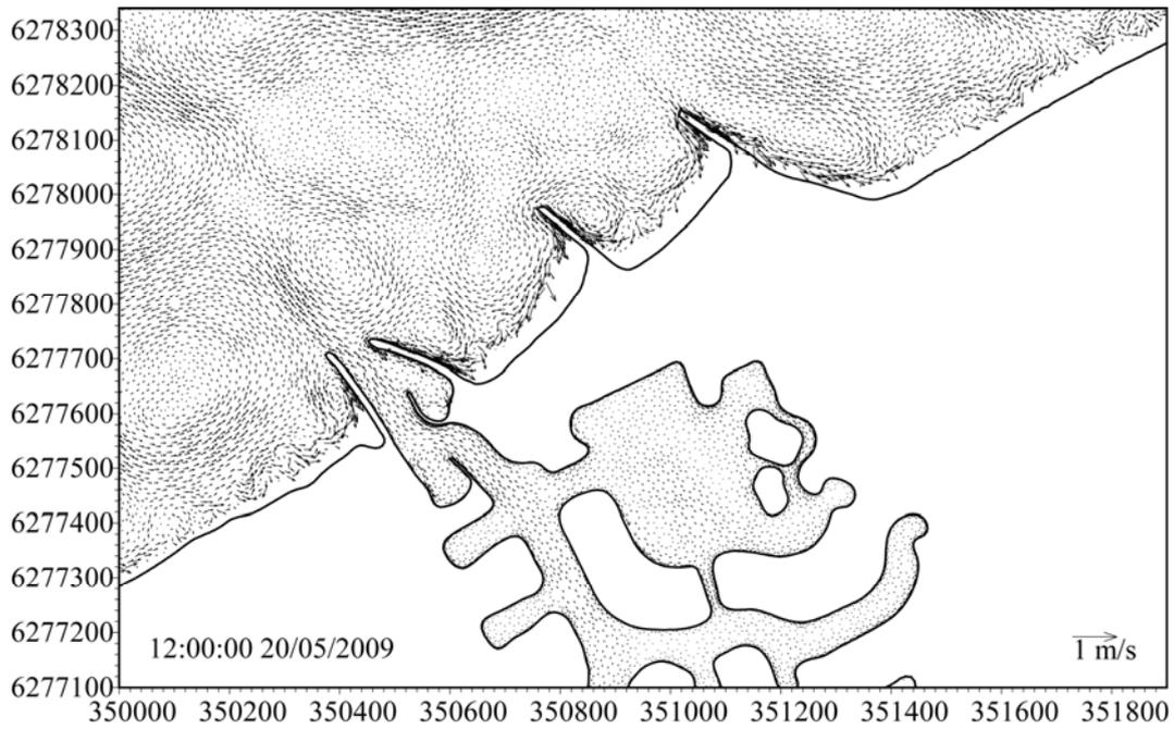
**Figure 4.9** Predicted velocity vectors in the vicinity of Port Geographe at the beginning of storm event (1200 hrs, 20 May 2009).
