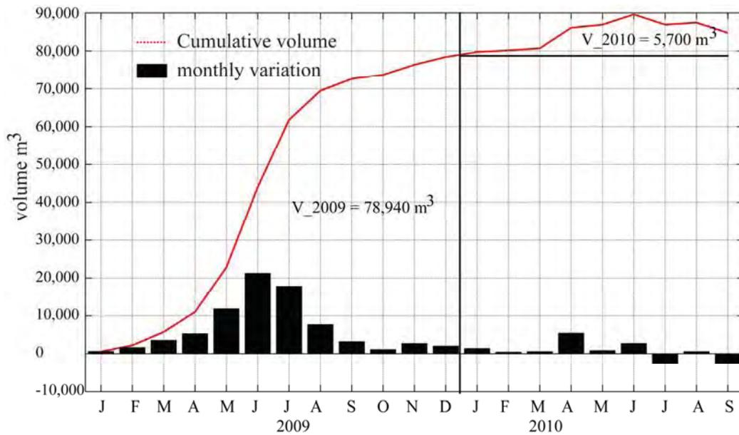
**Figure 4.19 Predicted monthly sand accretion (black bars) and cumulative sand volume (red line) from January 2009 to 30 September 2010 along the western side of Port Geographe.**
