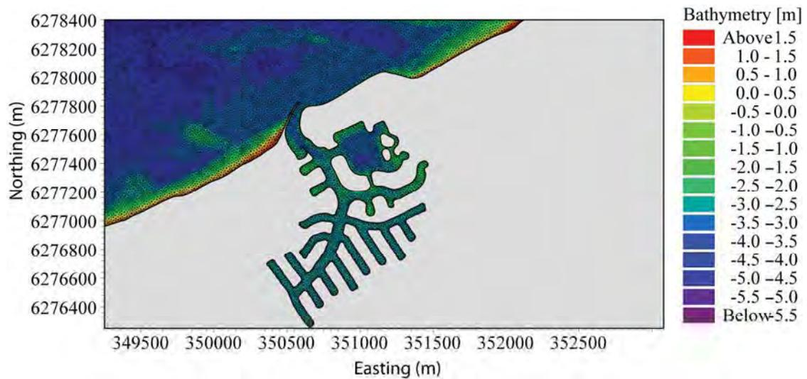
**Figure 4.70 Mesh grid and initial bathymetry in the vicinity of Port Geographe for Scenario 6 including all inner canal segments.**
