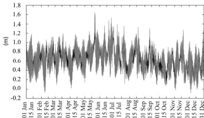
**Figure 2.6 Open boundary water level forcing data in 2009, from the Bunbury tide gauge (Source: Western Australian Department of Transport).**
