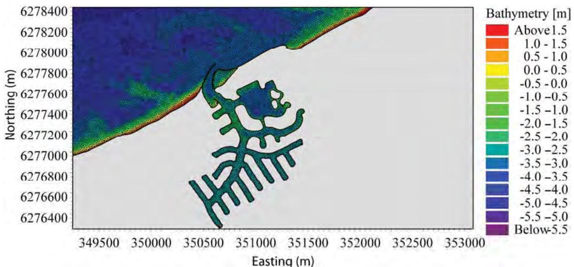
**Figure 4.86 Mesh grid and initial bathymetry in the vicinity of Port Geographe for Scenario 8 including proposed lagoon and all inner canal segments.**
