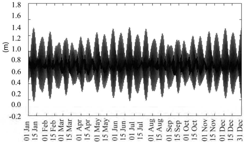
**Figure 2.7 Tidal water level variation in 2009 extracted from the Bunbury tide gauge records. (Source: Western Australian Department of Transport).**
