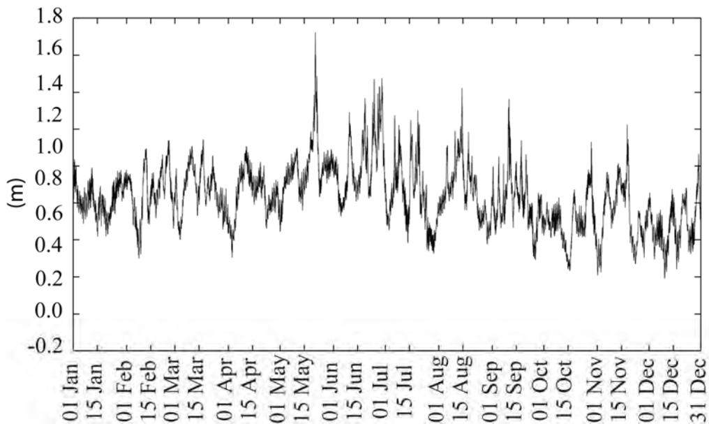
**Figure 2.8 Residual sea level variation in 2009 extracted from the Bunbury tide gauge record.**
