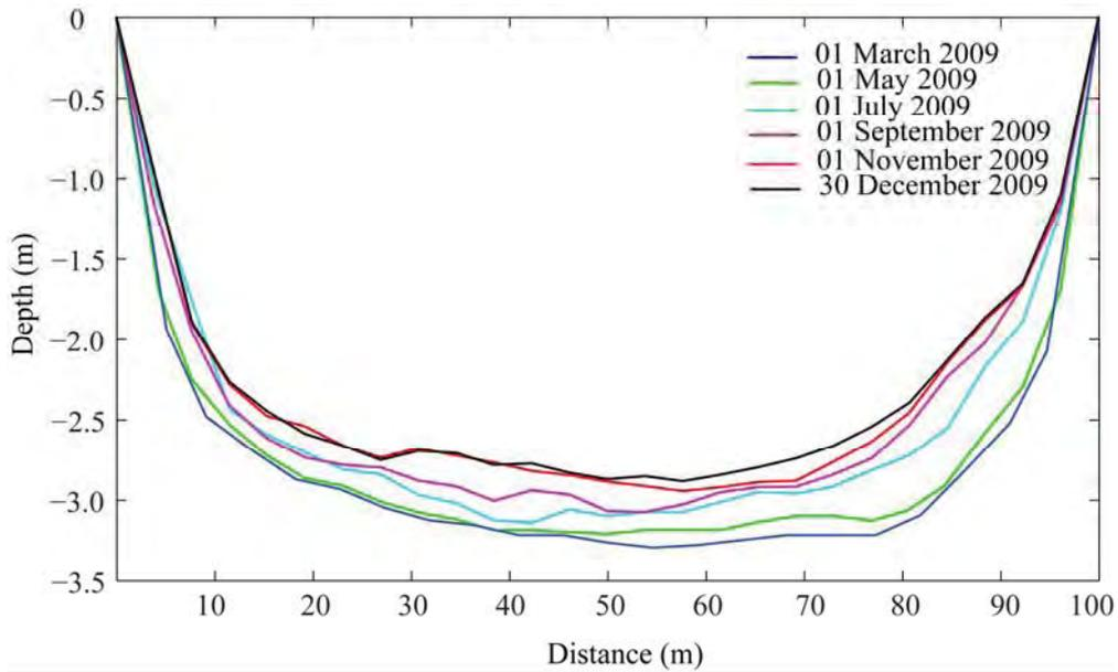
**Figure 4.72 Predicted bed levels across the entrance canal (section x-y) of Port Geographe for Scenario 6 from 1 March to 30 December 2009.**
