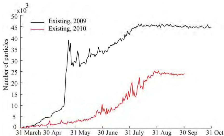
**Figure 4.24 Comparison of the cumulative number of particles, representing seagrass, at the western beach, Port Geographe in 2009 and 2010 with current configuration.**
