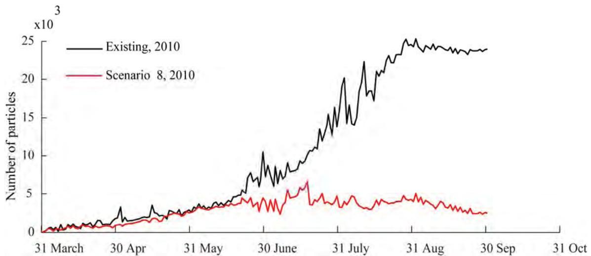
**Figure 4.100 A comparison of Scenario 8 and existing condition predicted cumulative number of particle (seagrass wrack) at the western beach, Port Geographe for 2010.**
