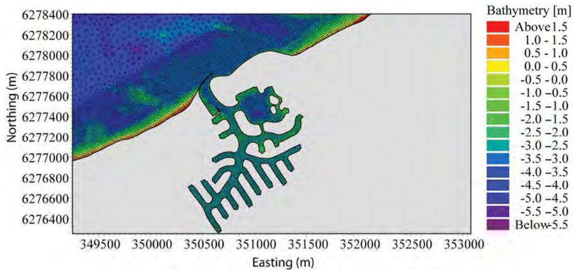
**Figure 4.27 Scenario 2 mesh grid and initial model bathymetry.**
