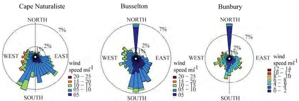
Figure 2.14 Wind rose diagrams at Cape Naturaliste, Busselton and Bunbury based on meteorological station data in 2009.
