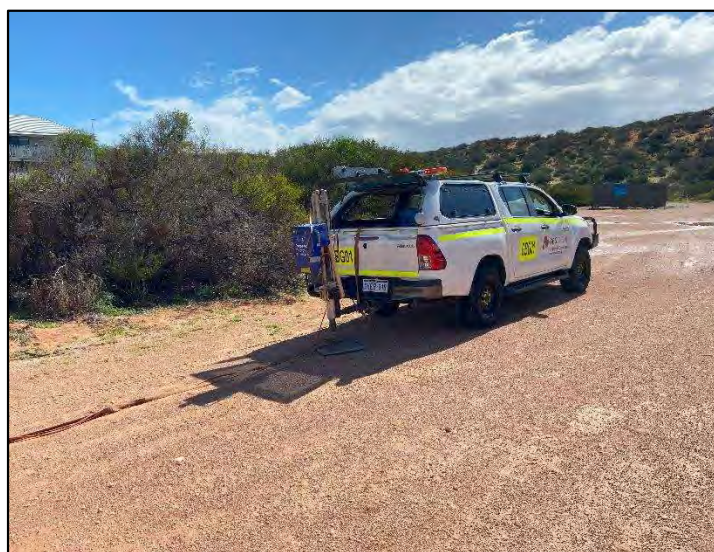
Figure 4: MASW data acquisition using a seismic streamer and AWD.
