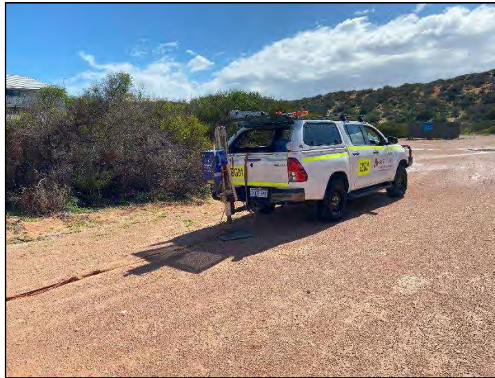
Figure 3: MASW data acquisition using a seismic streamer and AWD.
