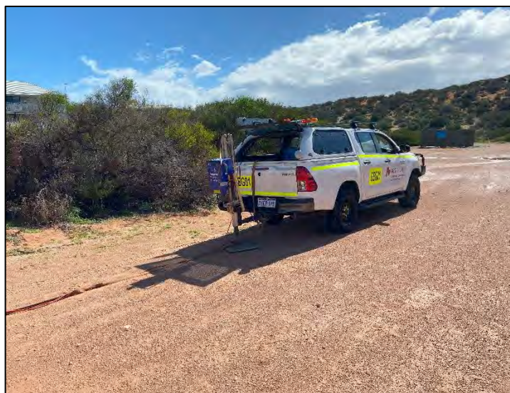
Figure 5: MASW data acquisition using a seismic streamer and AWD.
