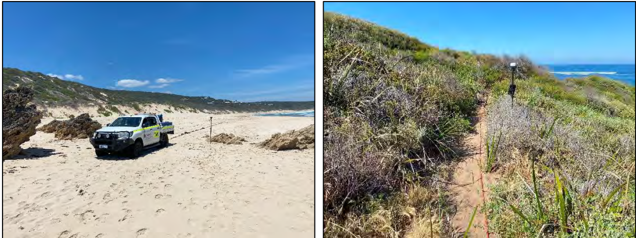
Figure 3: MASW data acquisition using a seismic streamer and AWD (left) or sledgehammer (right).
