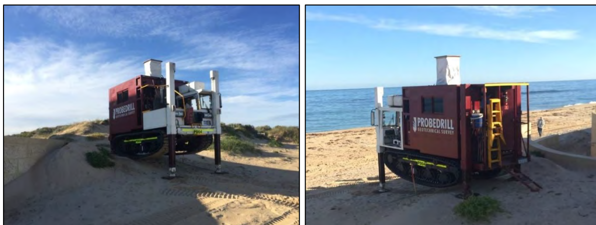
Figure 4: CPT data acquisition during a previous coastal investigation.
