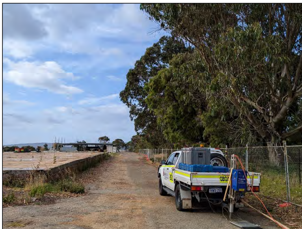
Figure 3: MASW data acquisition using a seismic streamer and AWD inside the old Albany woolstore
