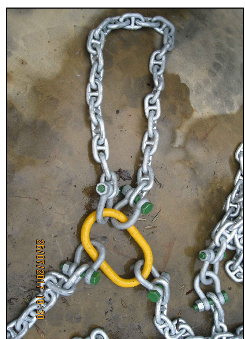
1 DETAIL - JUNCTION OF 2 LEGS (6 No. INCLUDING 1 SPARE) 8-1 NTS
